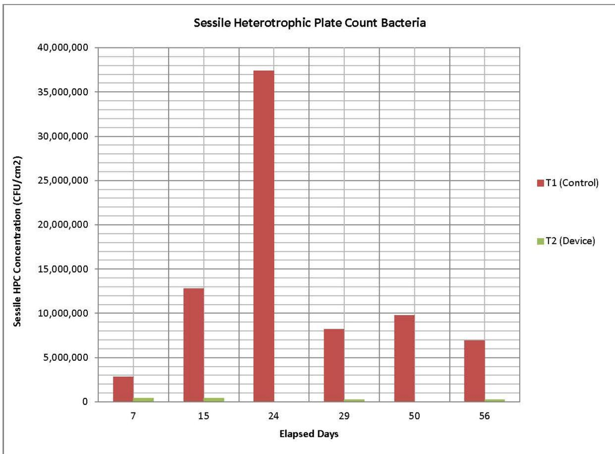
Sessile HPC concentrations in T1 (Control), and T2 (Device). The Day 50 sampling coupon for T2 (Device) was damaged and was not processed.
