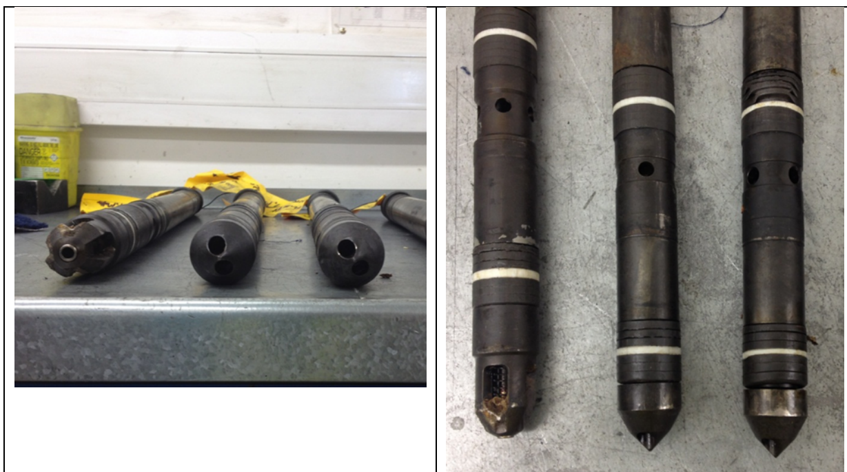
Figure 5. Gas Lift Valves retrieved from well under test showing no mineral scale deposition
