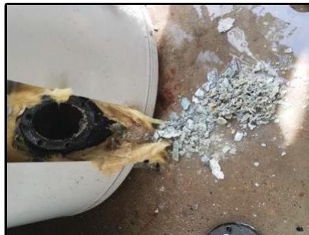
The heaters not treated with Flow-Tech had typical hard scale that needed to be manually broken off.
