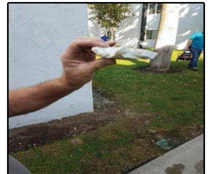
The heaters not treated with Flow-Tech had typical hard scale that needed to be manually broken off.
